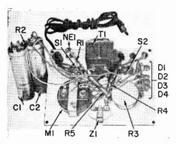
Although parts location is not critical for proper operation of the unit, builders will find it difficult to squeeze parts into the plastic case if they ignore author's layout.
