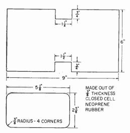
Dimensions for the rubber traction pads used to mount 6-volt battery on air tanks.
