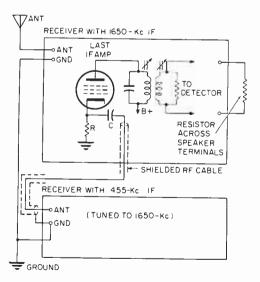
resistor should have the same value as the speaker impedance. Tune the second receiver to 1650-kc and tune in the stations with the first receiver. The audio volume control of the first receiver will have no effect. The RF gain controls of both receivers can be varied to get the required gain.
