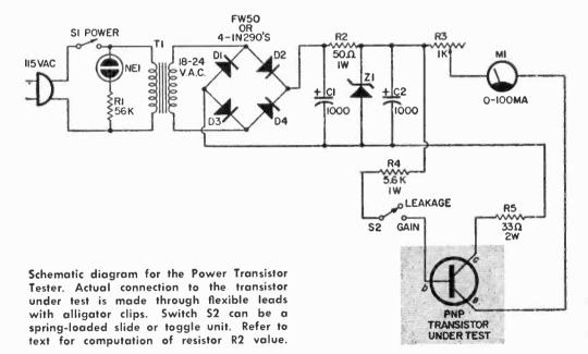
transformer used in our tester was salvaged from a piece of Minneapolis-Honeywell equipment although any transformer with a secondary of 18 to 24 volts, rated for a current of at least 200 ma. can be used. In order to determine the resistance of R2, the Zener current limiting resistor, for a different secondary voltage use the following equation.
