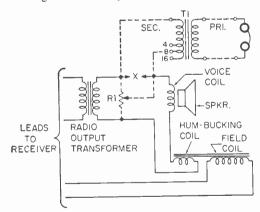
matic diagram. Connect the headphones across its primary (high impedance side). The transformer type suggested has three taps. Try the 4, 8 and 16 ohm taps and use the one that gives best results. The purpose of the added transformer is to step up the audio voltage. To use the speaker, turn the potentiometer fully one way. Midway, both the headphones and speaker will operate (at reduced volume). When fully turned the
