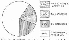
Fig. 2. Breakdown of the fundamental frequency and harmonics in a violin's sound.
