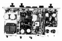
Two large printed circuit boards contain most of the components in the KP-70 preamp.
