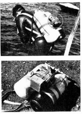
Six-volt battery pack is strapped to diver's air tanks (top photo). Aqua-Com is attached to diver's belt except in bottom photo where it can be strapped to tanks.
