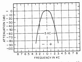
Fig. 2. Bandpass of mechanical filter is  $onl\hat{y}$ 5 kc. wide at 60 db down. Note steep sides of curve block out side band pickup.
