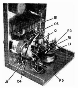
R3 is mounted to the cabinet with an L bracket made from straightened cable clamp.
