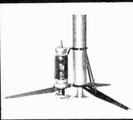
Multivibrator, a biological Mars probe, is designed to seek out basic carbon compounds of life. Left, unit and container; below, fluorescent light tes: chamber.
