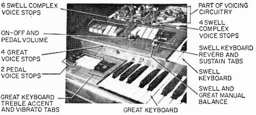
Fig. 9. Photo of left side of keyboards shows complex switching used to get voicing.
