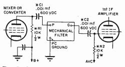
Fig. 5. Circuit modification for mechanical filter—\* indicates added circuit components.
