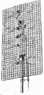
Fig. 3. Four individual bays are stacked one on top of the other for greater gain.
