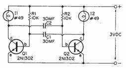
Be sure to connect positive leads of electrolytic capacitors to Q1 and Q2 collectors.
