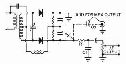
If your tuner does not have a multiplex jack, you will have to provide your own by tieing into the FM tuner audio output circuit immediately before the de-emphasis network. How it is done schematically is shown above for the ratio detector and below for the discriminator detector. Actual detector circuits may vary from unit to unit, but R1-C1 network is always used to provide de-emphasis effect.
