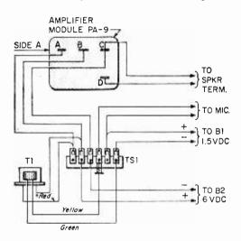
The pictorial diagram shown above should be used only if the terminal configuration in the amplifier module you purchase is identical with the diagram. Otherwise, follow the diagram supplied with the unit. Although the module may appear to be different, it is an exact electrical replacement.
