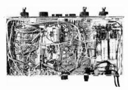
Even though most components are on circuit boards, considerable wire and shielded cables are used to interconnect all audio circuits.
