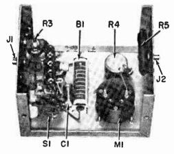
Inside view of the Tape Tester is uncluttered and easy to wire. Note that VU meter circuit is physically isolated from the oscillator.
