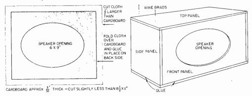
Speaker Grille Detail Drawing—Using materials found at home can reduce cost to zero.
