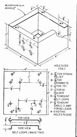
Detail drawings above provide the information necessary to pre-drill the aluminum case. Belt loops made from wire hangers.
