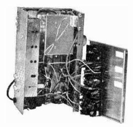
How does KLH make it so small? The multiplex circuit is mounted on the top plate and folds over the chassis when the plate is installed. Note the extensive use of shielded cables and cover-plate metal shields—neatness helps.
