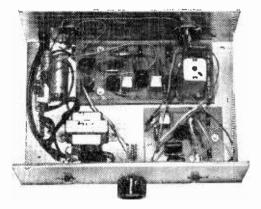
Semiconductor circuit offers long term troublefree performance. Two jacks on rear panel connect to FM tuner and amplifier input.
