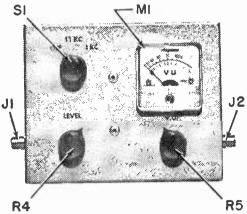
Front panel view of Tape Tester showing location of controls, VU meter and interconnecting jacks. Decals add pro look to assembly.
