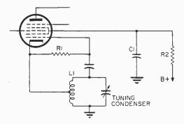
range. The trouble is usually due to a defective converter tube, change in the value of the oscillator grip leak (R1) or in the value of the screen voltage dropping resistor (R2). It could be that by-pass capacitor C1 may be leaky causing the screen voltage to drop. Try a new grid leak (R1) of the same value as the original. If that doesn't do it, change R2 and C1. Sometimes the oscillator coil (L1) absorbs moisture and its Q is lowered. Try drying it out by exposing it to an infrared lamp.
