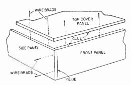
Cabinet Detail Drawing #1—Cover for unit is glued—brads hold pieces while glue sets.
