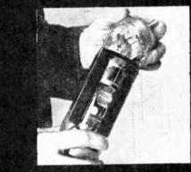
Inner sphere in Advanced Mariner lander contains scientific payload and communications, and is protected by impact crush-up case.
