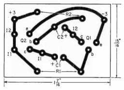
Detailed diagram of underside of printed circuit board—be sure to copy to scale.
