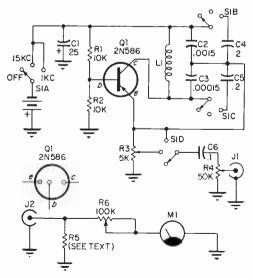
Schematic diagram for the Tape Tester—keep \$1 set at off during playback of test tape.
